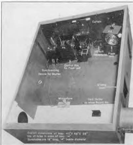
FIGURE 3. Interior of the box, showing Microflash, microphone, synchronizer, and other equipment.
