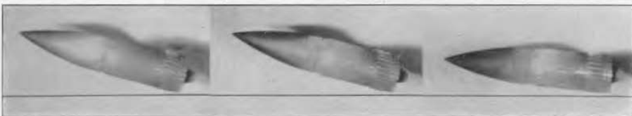
FIGURE 7 (below). These three rounds show excessive yaw. The line below them indicates the line of flight.
