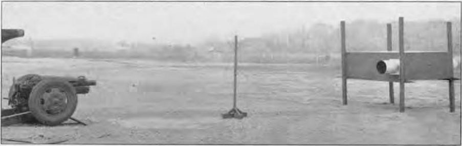
FIGURE 2. Arrangement of equipment for photographing projectiles 100 feet from the gun. At the left is the gun, at the right the box through which the projectile passes to be photographed. On the post between the two is the pressure switch which opens the shutter when the projectile passes.
