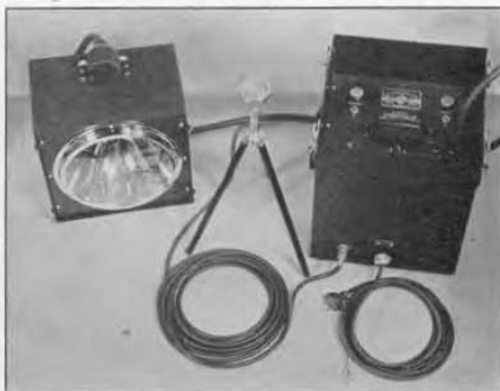
FIGURE 5. View of the Microflash Unit, consisting of light source, power supply, microphone, and connecting cables.
